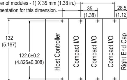
NOTE: All dimensions are in mm (inches). Hole spacing tolerance:  $\pm 0.4$  mm (0.016 in.)
